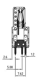
Material: Contact Solder Pin: Copper, Tin Plated Retention Ring: Stainless Steel Insulating Body: Polyamide, UL94V-0, Green Electrical Voltage Rating: 600 VAC Current rating: 41 AMPS Withstand Voltage: 1500 VAC, Test time 60 seconds Mechanical -40°C to +115°C Operating Temperature: -40°F to +240°F Soldering Temperature: 260°C, 500°F for 5 seconds max. c Dus Safety Approval:
