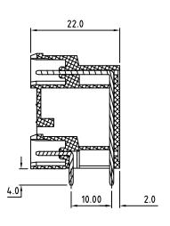
Material: Contact Solder Pin: Copper, Tin Plated Insulating Body: | Polyamide, UL94V-0 Flange Nut: M2.5, Brass Electrical Voltage Rating: 300 VAC Current rating: 20 AMPS Withstand Voltage: 1500 VAC, Test time 60 seconds Mechanical -40°C to +115°C Operating Temperatures -40°F to +239°F Soldering Temperature: 260°C, 500°F for 5 seconds max. c Rus Safety Approval:
