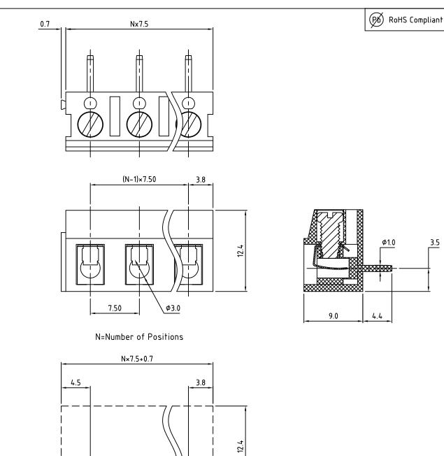
Material: Contact Solder Pin: Brass, Tin Plated Wire Guard: Stainless Steel Screw: M3, Steel, Zinc Plated, "-" slotted Insulating Body: | Polyamide, UL94V-0 Electrical Voltage Rating: | 300 VAC 15 AMPS Current rating: Withstand Voltage: 1500 VAC, Test time 60 sec Wire Range: 14-22 AWG Mechanical Torque: 3.5 Lbs-in. Max -40°C to +115°C Operating Temperature: -40°F to +239°F
